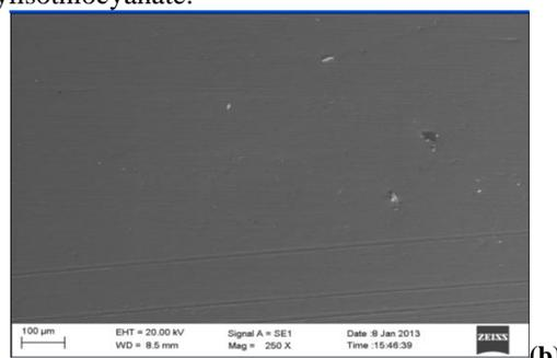
**Figure 9(b):** SEM image for Al metal in H<sub>2</sub>SO<sub>4</sub>( pH= 2.3)+CPSE
